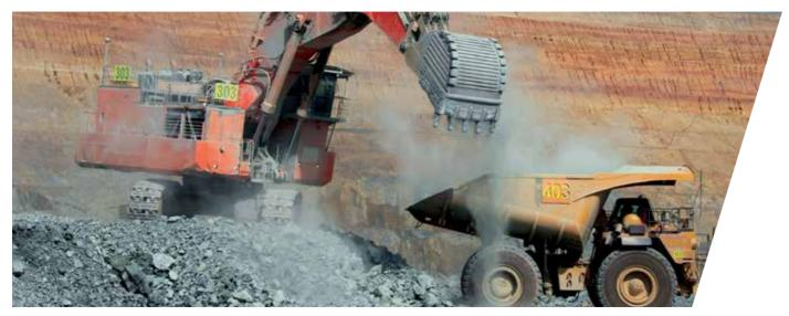
5 position excavator bucket working in a gold mine in Australia.
