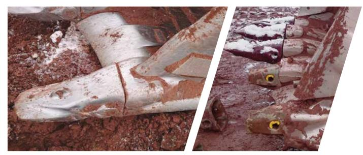
MTG Systems StarMet Cast Corner adapter in abrasive applications.
