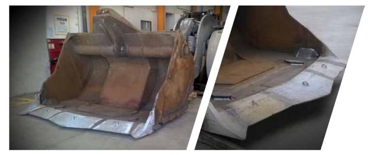
Bucket with LHD Lip System in underground copper mine.
