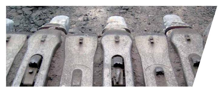
Close-up of a MTG Systems StarMet Rope Shovel adapter with a conventional locking system.
