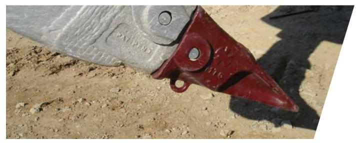
MTG Systems tooth for bulldozers working in Spain.
